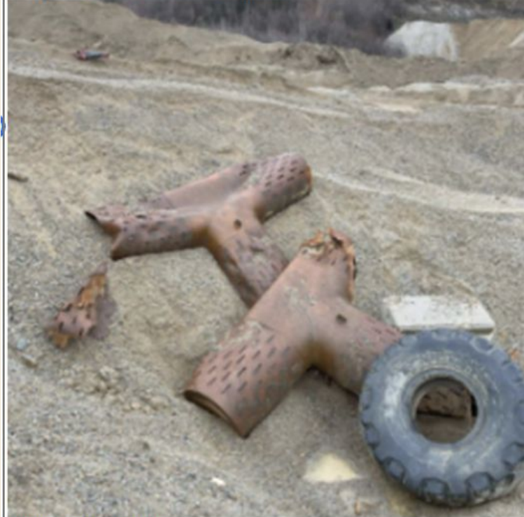
Figure A.1.40: 450-mm screened-steel pump intakes
